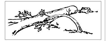
5 Take the utmost care when cutting through branches or logs that are in tension. A log or branch that is in tension can suddenly spring back into its natural position before or after you cut it. If you stand on the wrong side or start cutting in the wrong place it may strike you or your chain saw. This could make you lose control and cause a serious accident.
